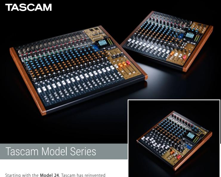
Starting with the **Model 24**, Tascam has reinvented its legacy, one of its classic lineups, infused with the latest audio technology. Model Series mixers let you directly record to an SD card, 24, 16 or 12 tracks simultaneously in 24 bit / 48 kHz, and punch in/out eight tracks at the same time. You can stream playback audio from your smartphone to the mixer and connect to your DAW via USB.
