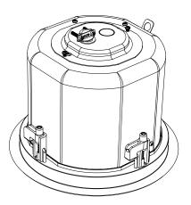
Undo the two screws that secure the protective plate on the top of the back can
