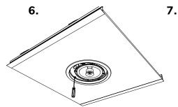
Carefully tighten the locking tabs using a suitable Philips screwdriver until they are tight. Do not overtighten
