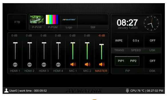
The information of user name, working time, USB connection, CPU working temperature, system time keeps displaying in the bottom of the Status/Menu page.
