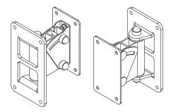
In applications where precise alignment and tilting to the audience areas required, this swivel and tilt mount is used. It supports a single P10 loudspeaker.
