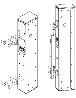
Note: If the lock washers ("RIPP LOCK") are not used at all or not sufficiently tightened, the ball impact safety certificate according to DIN 18032-3 is invalid. So please always ensure correct assembly based on these instructions.
