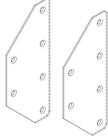
2.3 Swivel and tilt bracket for one loudspeaker
