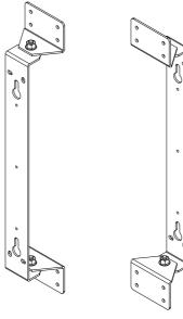
The mounting of a single P10 speaker can be implemented using the U-bracket included as standard.
