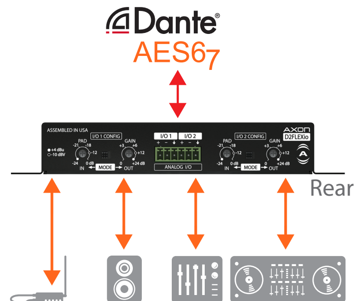
Application illustration only, maximum of 2 channels of analog I/O connectivity
