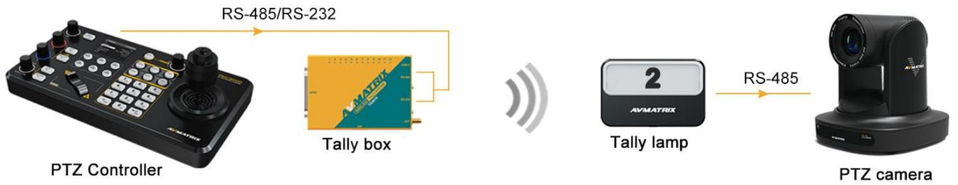
Wireless remote control of the PTZ camera can be achieved with the TS3019's serial pass-through function.
