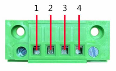
Euroblock: Connect the positive pole to 3 or 4, and the negative pole to 1 or 2.
