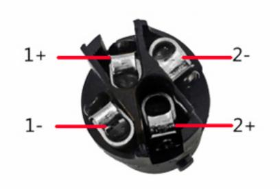
Ohm plug connection method: Connect the positive pole to 1+, Connect the negative pole to 1-, 2+ and 2- are not wired.
