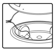
6. Attach signal wire to wire leads. Use wire nuts provided. For added water proofing, grease caps are recommended.
