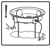
4. Place speaker base into hole in ground with the top rim of the base at ground level. Back-fill dirt in to hole, packing the dirt firmly. For added security, cement security brackets into ground.
