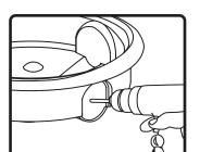
1. If needed for daisy chaining drill speaker base and install second liquid-tight strain relief (not included).
