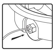
3. Thread signal wire through liquid-tight strain relief and tighten seal.
