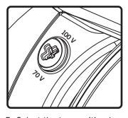
5. Select the tap position by removing the rubber plug to access rotary switch. Switch is preset to maximum tap setting in 70.7 V mode (64W XT850, 32W XT550). Select desired setting and reinsert rubber plug.
