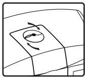
11. Position speaker at the desired angle and secure with the clamp knob. As a security feature, an included 5 mm Allen hex key is required for loosening the clamp knob and readjusting the speaker position angle.
