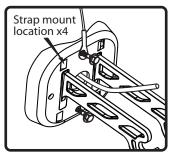
4. Thread safety cable (included) through mounting screw and securely fasten mounting plate to surface (user must supply fasteners). Mounting bracket may also be strap-mounted to pole or appropriate anchor point. The max. strap width is 0.5 in / 12.7 mm.
