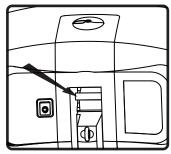
10a. When mounting the speaker, ensure that the mounting rod in the speaker securely engages with the mounting prongs on the bracket arm.
