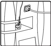
8. Clip snap-link safety cable to eyebolt on back of cabinet.
