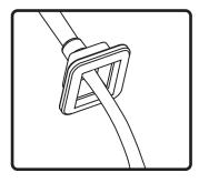
5. Slip terminal weather boot over signal wire. For environmental applications, put sealant around nipple and base when installation is complete.
