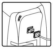
7. Insert four-pin Euroblock connector into jack on rear of speaker. Connectors are keyed for polarity.
