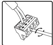
6. Connect signal wire to four-pin Euroblock plug. Use inside positive and negative inputs for signal wire input. For daisy chaining, use outside positive and negative terminals to connect additional speakers. Tighten unused terminal screws.
