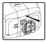
10b. When properly inserted, bracket arm prongs will be fully engaged with the mounting rod in the speaker cabinet.
