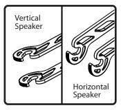
3. For proper bracket and plate orientation, pay special attention to the prongs on the bracket arm and ensure that they point toward the direction of the desired speaker position.
