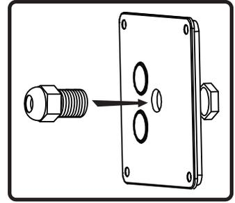
4. If being installed per EN54-24 regulations or in instances where a water tight strain relief bushing is necessary, attach the included strain relief bushing to the back plate. If it is not required, skip this step.
