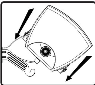
9. Tilt speaker 45° (grille up) and slide on to bracket.
