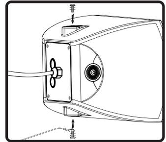
8. Select desired location for safety cable install using U-bracket mounting screw. If mounting speaker horizontally, attach safety cable to one of the vertical mounting points and vice versa.
