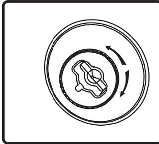
6. Select the tap position by rotating the rotary switch located on the back of the speaker to desired setting. The switch is preset to the maximum tap setting in 70.7 V mode (32W for the SM52-EZ[-WX] and 64W for the SM-82-EZ-II[-WX]).
