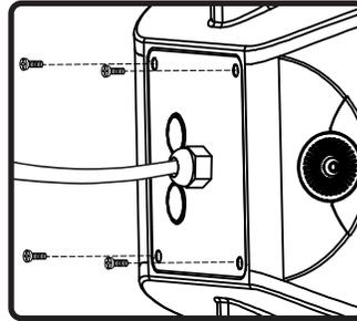
7. Install back plate and secure with included fasteners.
