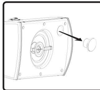
If used indoors, remove the grille and take the plug out of the port for greater bass output. Port must remain plugged to maintain IP65 rating in outdoor use.
