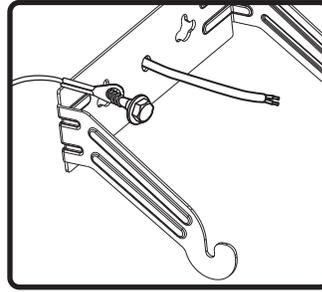
3. Mount u-bracket with clamping slots pointing upward. Securely fasten mounting bracket and safety cable to surface (user must supply fasteners). **Note:** The safety cable will attach to one of the speaker's unused mounting holes using one of the included mounting screws.
