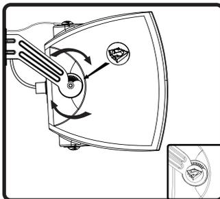
10. Aim speaker and tighten u-bracket screws. Once tightened down, place the screw caps on the screws. Done!
