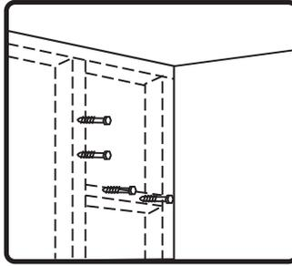
2. Choose a secure mounting surface with sufficient strength to reliably hold the speaker. The speaker may be mounted in either the vertical or the horizontal position with the same U-bracket.
