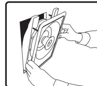
**5.** Insert speaker in to hole (bottom first) with mounting bar on inside of wall.
