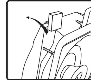
**3.** Remove styrofoam inserts between mounting bars and speaker baffle. (4x)
