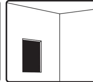
**2.** Use provided cut out template to make hole. Use Rotozip or other tool to cut hole in wall. Hole size, 7.5" x 10.75"
