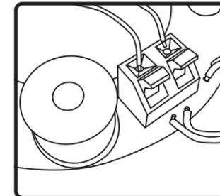
**4.** Connect speaker wires to terminals on rear of speaker.
