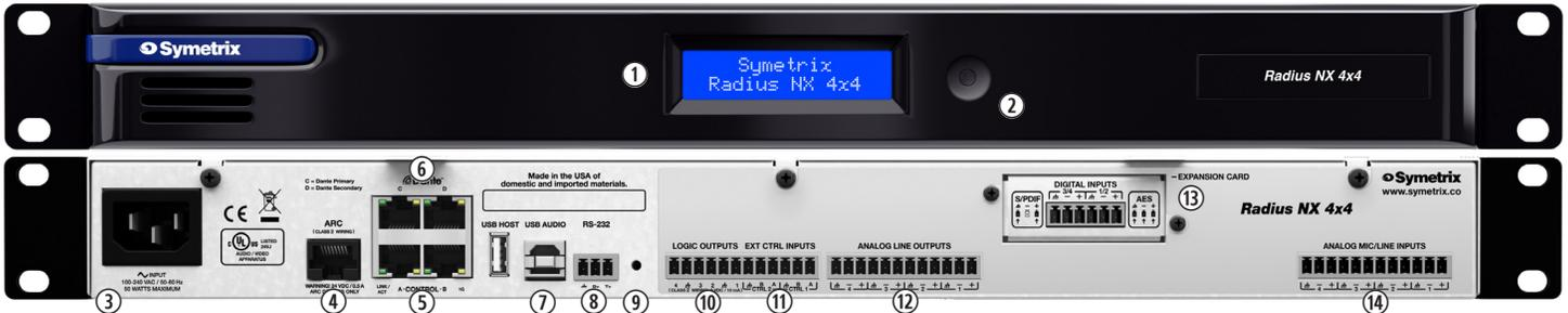
① **Display:** Shows either an overview of system parameters or level meters for analog inputs, analog outputs, USB I/O, and expansion card I/O. The overview contains limited information such as IP Address, DHCP Status, and communication LEDs for Ethernet, Dante, and ARC. A short button press moves between the overview and input/output meters. The meters are scaled from -72 dBFS to 0 dBFS. Each segment represents 12 dB. If the signal reaches clipping, the meter will get wider.
