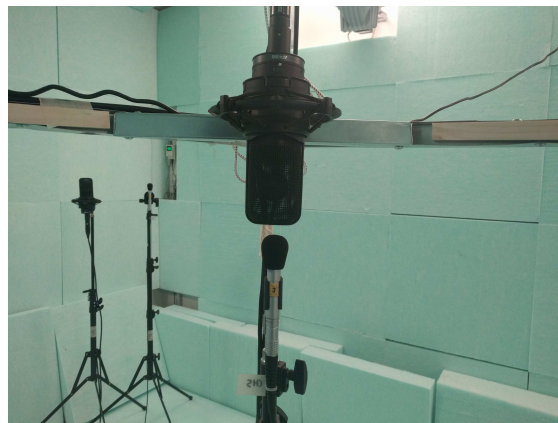
Figure 5: Detail with one of the B&K 4190 microphones used as reference and one of the recording microphones AT 4050.
